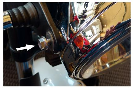
② Use 12mm socket to loosen one of the hex screws that holds the headlamp in place. Do not remove all the way. (TIP! this will be easier if you have a friend to help hold the headlamp in place).
