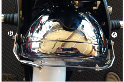
(A) Install one arm of the AltRider headlight guard with the screw you just removed. Leave this screw loose for now. (B)Then completely unscrew the first side and finish the installation of the headlight guard. Tighten both screws. Check headlamp aim in accordance with manufacturer's instructions.
