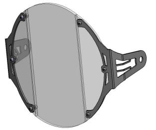
Assemble polycarbonate lens to stainless frames. Peel protective film back from polycarbonate lenses. Use T10 torx and 5.5mm nut driver to attach lenses to frames. Place M3 torx screws and washer against polycarbonate, and with M3 locknut on back side agains stainless steel frame.
