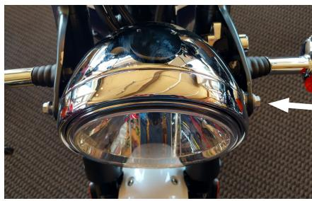
3 Loosen the screw on the other side and remove completely. Careful not to lose any spacers or washers (varies by model).
